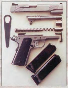
Here, the fieldstripped SW1911 is seen. The pistol comes with two eight-shot magazines and a barrel-bushing wrench.
